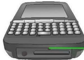
Insert a pin into the recess to trigger the hard reset button
